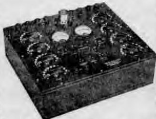
Figure 1. The Type 361-A Vacuum Tube Bridge Manufactured by the General Radio Co.
